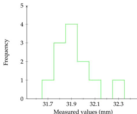
Figure 1: Data obtained when measuring the length of a piece of wire
