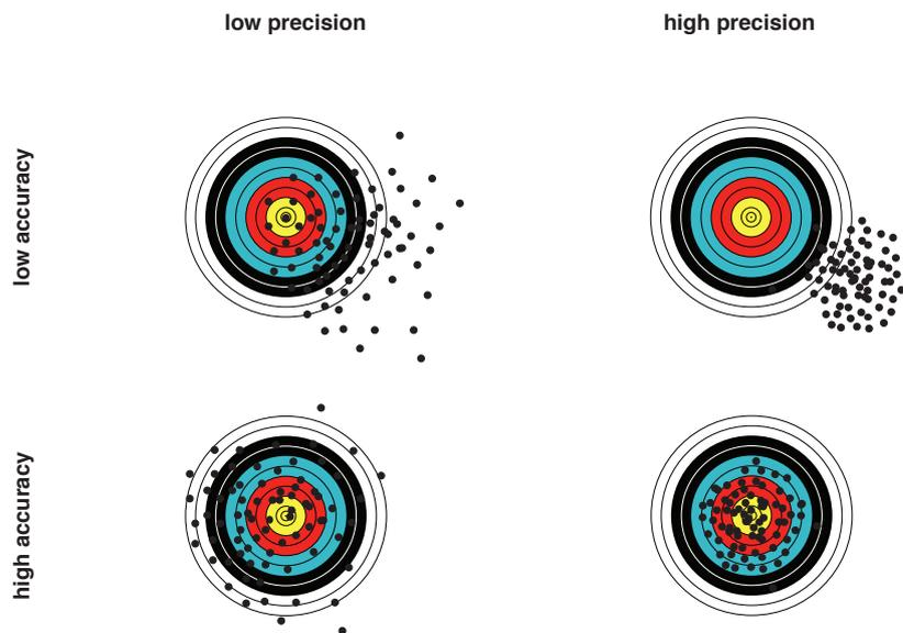
Figure 2: The difference between accuracy and precision.
